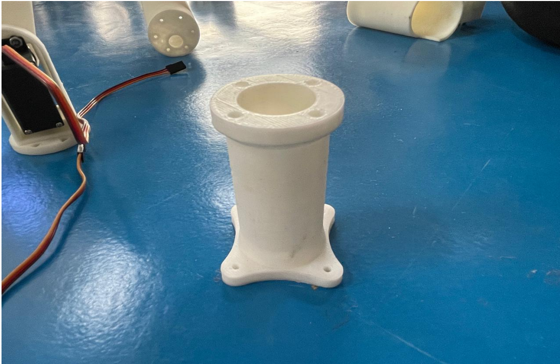
Photograph 5: 3D Printed Cam tube.
