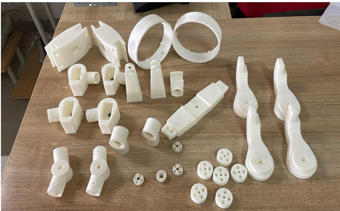
Photograph 6: 3D Printed Parts of Robot.
