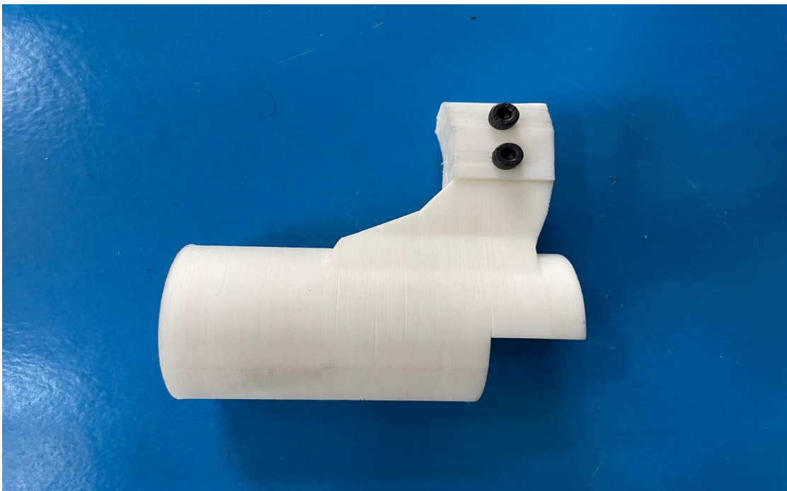
Photograph 4: 3D Printed Wheel joint.
